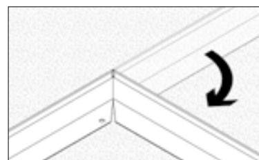
STEP 2 - Bend by hand (past the 90 then back for right angles) and perfect shape with rubber mallet.
